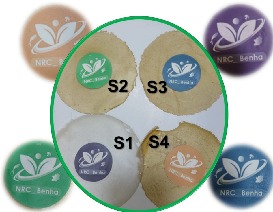
Fig. 4 Soluble starch films with different ratios of broccoli extract as substrate for printed edible labels
